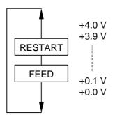
**NOTE:** If "0.0 V" is set, when the power is turned OFF then ON, the value "0.0 V" is returned to the initial value (1.0 V).
