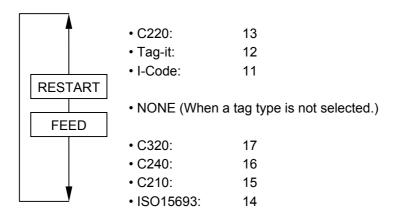
This setting will become effective after the printer power is turned off, and back to on. Only the tag types, which can be read/written by the modules set by the RFID module setting, are displayed.
