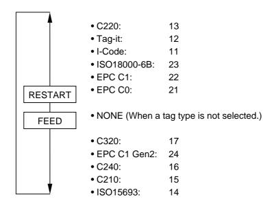
② When the RFID module type is set to "U2":
