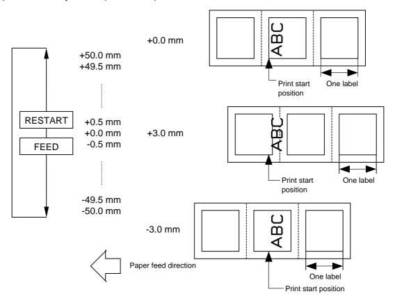
(2) Cut position (or strip position) fine adjustment (CUT ADJ.)
