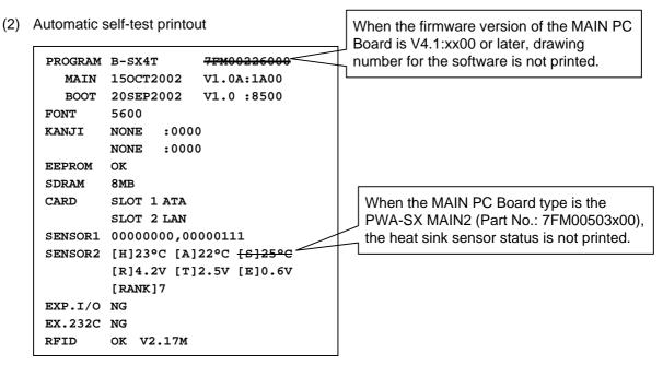
**NOTES:** 1. Print conditions: 87 mm of label length, thermal transfer/direct thermal print mode<sup>(\*1)</sup>, no sensor used, 6 ips/5 ips<sup>(\*2)</sup>, one sheet to print, batch issue, no driving of paper rewind motor
