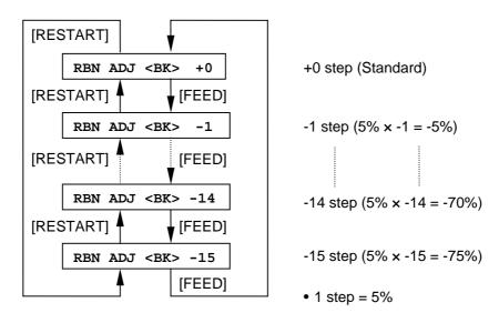
(8) Transmissive sensor manual threshold fine adjustment setting (THRESHOLD<T>)
