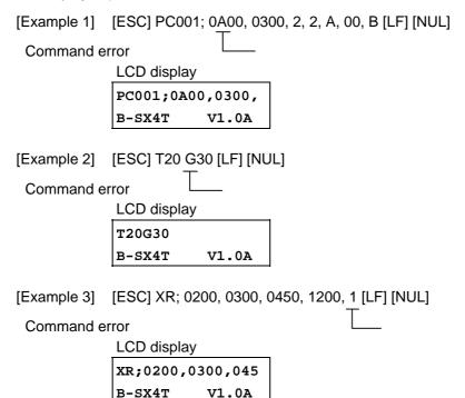
**NOTE 2:** When the command error is displayed, "? (3FH)" is displayed for codes other than 20H to 7FH and A0H to DFH.
