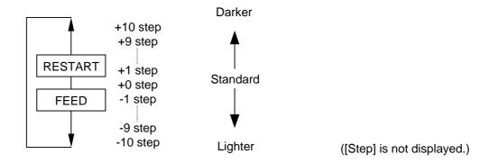
(6) Ribbon motor drive voltage fine adjustment setting (Rewind) (RBN ADJ <FW>)
