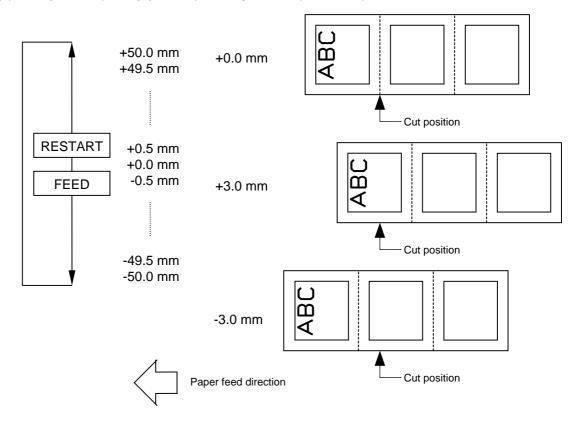
[Procedure for label having label pitch of less than 38 mm when the swing cutter is used]
