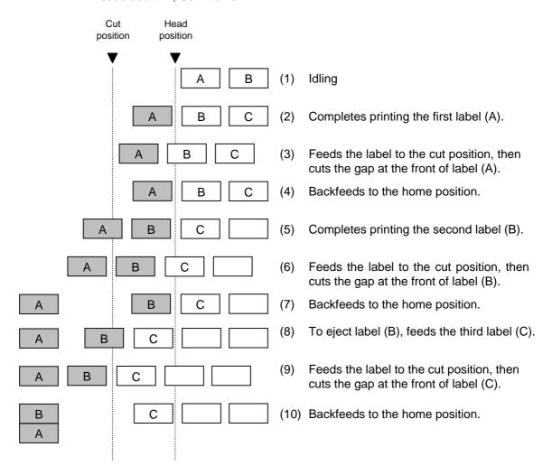
[Procedure for label having less than the min. label pitch for each issue speed when the rotary cutter is used]
