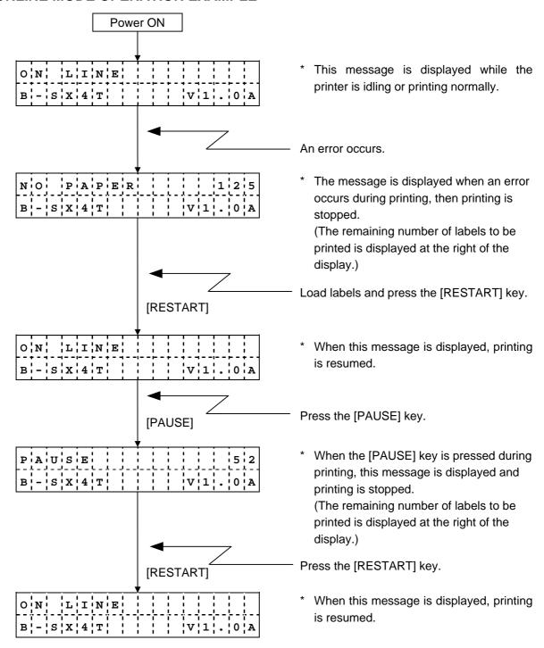
**NOTE:** [Remaining number of labels to be printed] = [Designated number of labels] - [Number of labels/tags normally printed before an error occurs or the printer stops temporarily]
