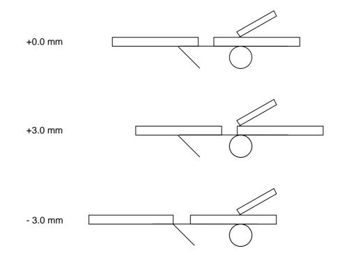
Printing in strip issue mode is stopped at the position where the distance from the middle point of the gap between labels to the end of the strip shaft is 4 mm, since the gap between labels is assumed to be 2 mm.
