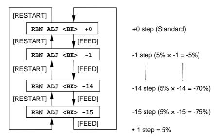
(7) Ribbon motor drive voltage fine adjustment setting (Back tension) (RBN ADJ <BK>)
