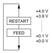
**NOTE:** If "0.0 V" is set, when the power is turned OFF then ON, the value "0.0 V" is returned to the initial value (1.4 V).
