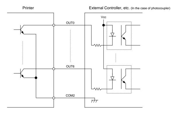
There are 7 output circuits, and each output is an open collector. The voltage of Vcc is  $24\ V$  (max.) while the drive current is  $150\ mA$ .
