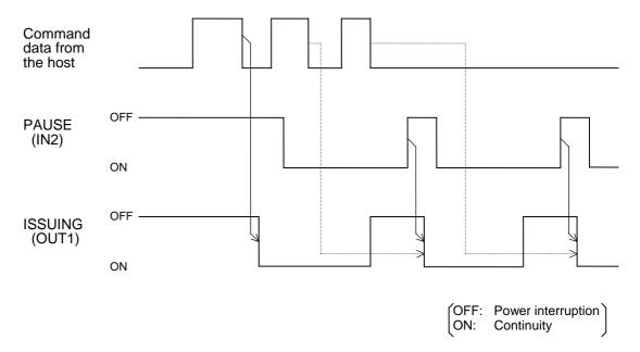
A pause state generated by the PAUSE signal cannot be cleared only by the [RESTART] key of the printer. However, the pause state, generated by the [PAUSE] key, can be cleared when the PAUSE signal goes from on to off.
