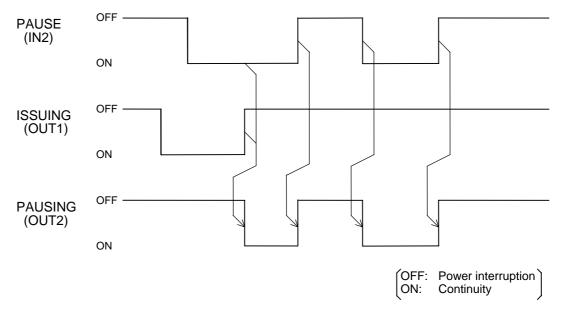
Even if the PAUSE signal is input during issuing or feeding, the PAUSING signal is not output until the issuing or feeding is completed.
