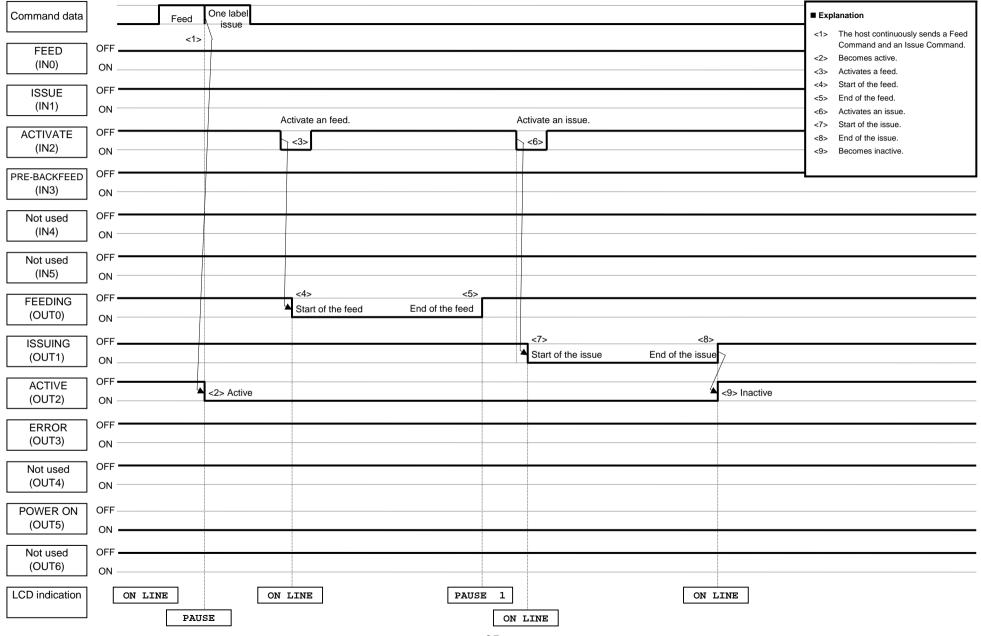
(4) When a feed is performed by the FEED signal during the active state.
