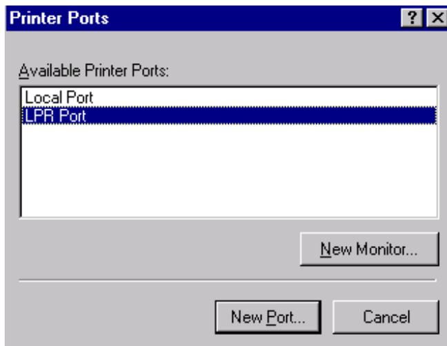
6. The Add LPR compatible printers box will then appear as shown in the following picture. Type in the IP address assigned to the print server in the **Name or address of server providing lpd** box.
