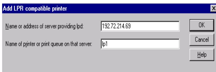
7. In the **Name of printer or print queue on that server** box, type in a printer name, for example, lp1. Click **OK**.
